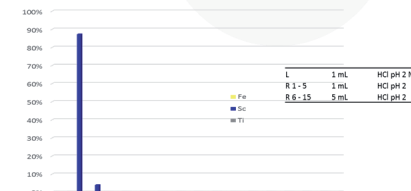
Fig. 8: Elution study Hydroxamate resin, 100 mg, load from 0.01M HCl, multielement solution (ME), fractions analysed by ICP-MS
